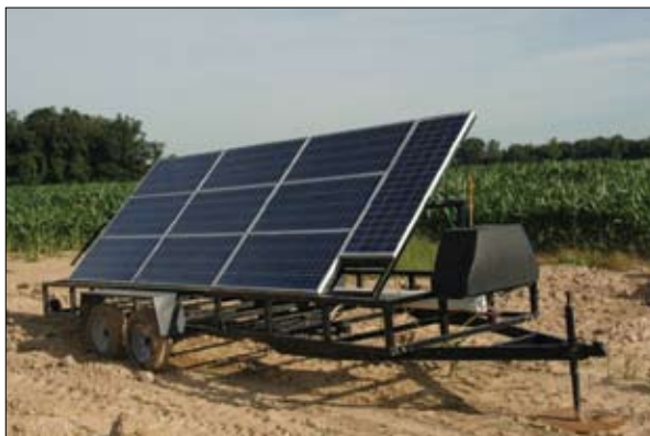
Movable Solar Panels
